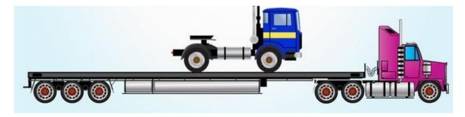
A van is the rectangular part of the truck. A truck may have a cab (shown on the flatbed) that attaches to a van, or it may be all in one piece, in which case it's called a straight truck. Vans are used to carry dry goods, like boxes of cereal, books, or toys.
